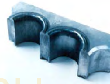
MOCK UP WELDING TUBESHEET: SB 443 TUBES: SB 444
